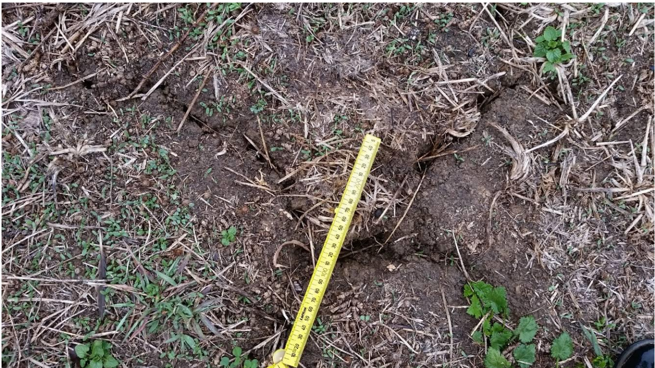
Photo 10 Cracks in hard-setting surface soils were observed across the site in sparsely grassed locations (HMC 2018).
